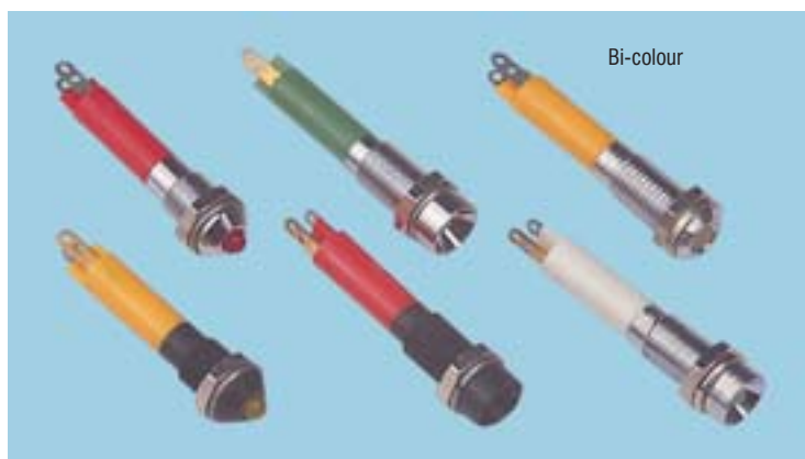
Prominent: Total L behind bezel=28.9 Recessed: Total L behind bezel=30.4 Flat-top: Total L behind bezel=32.4 All types: Bezel dia.=7, thread=M6x0.75, mounting hole dia.=6, tab connections=2x0.5, tinned tab indicates cathode (-), common cathode or bi-colour.
